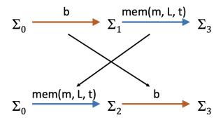
Shared variable m is always protected by lockset L thread t holds at least one lock in L during the access to m
