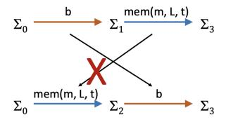
Shared variable m is always protected by lockset L thread t holds no lock in L during the access to m
