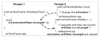
Assumption: *mOffset* and *mLength* are updated atomically wrt thread 1 Lack of synchronization  $\Rightarrow$  thread 1 read inconsistent value
