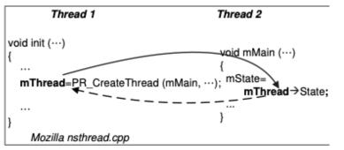
Thread 2 should not deref. **mThread** before Thread 1 initializes it Pattern:
